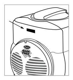
The left LED is red and lights to indicate that the unit has power. The right LED is green and lights when the unit is set to ultrasonic sound output.
